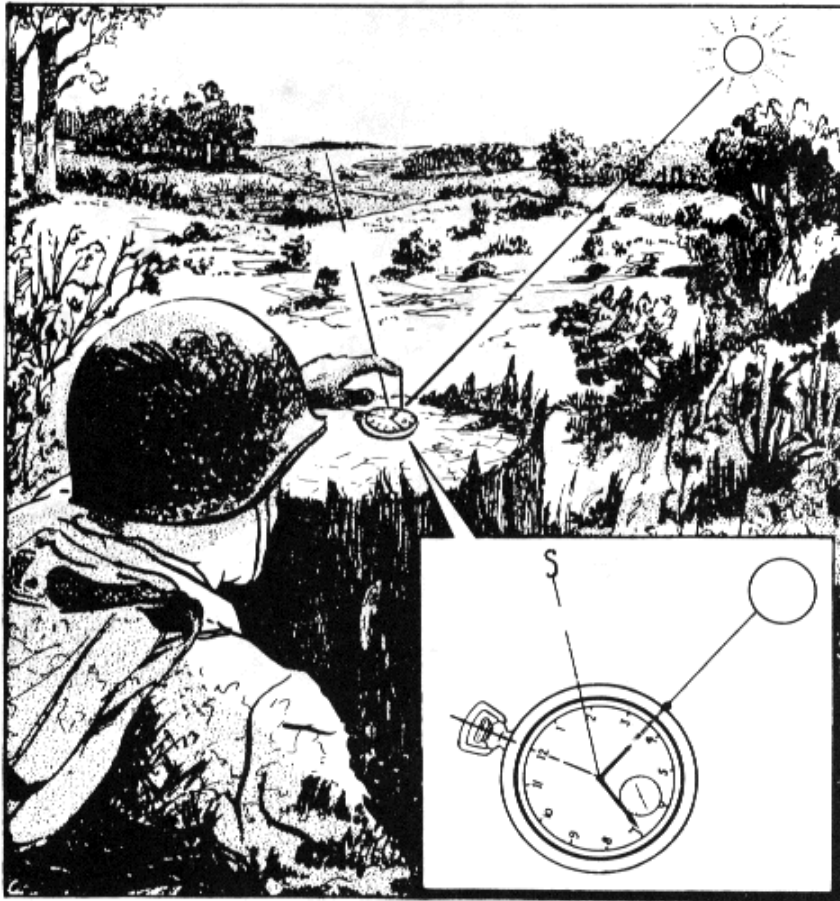
Figure 9. Sun and watch method of determining direction.
